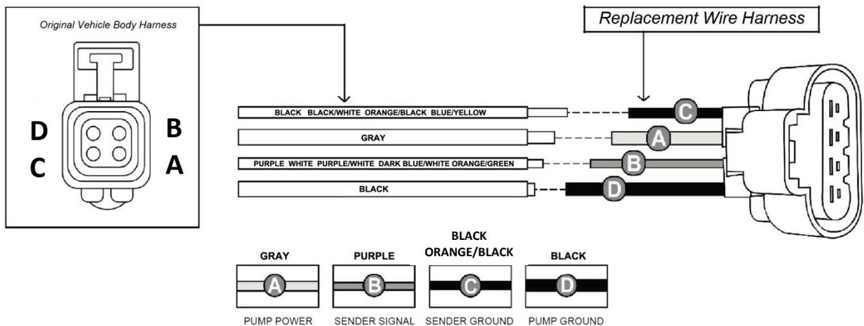
*NOTE: Crimped connectors must be staggered to allow the harness to fit inside the vehicle wire sleeve.*
